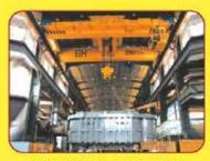
2001 x 25m Span x 30m Height Overhead Cranes For Lifting of Generator / Turbine In Tandem (Power Sector)
