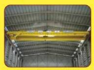
50T x 40m Span x 30m Height Double Girder Overhead Traveling Cranes (Oil & Gas)
