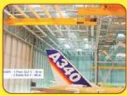
9T x 68m Span x 20m Height Underhung Crane (Aerospace)
