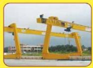
10T x 30m Span + (6m+6m) Cantilever C-Shaped Gantry Cranes (Steel)
