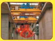
Cranes Fitted with Orange Peel Grab Waste Management Automated System (Waste Treatment Plant)
